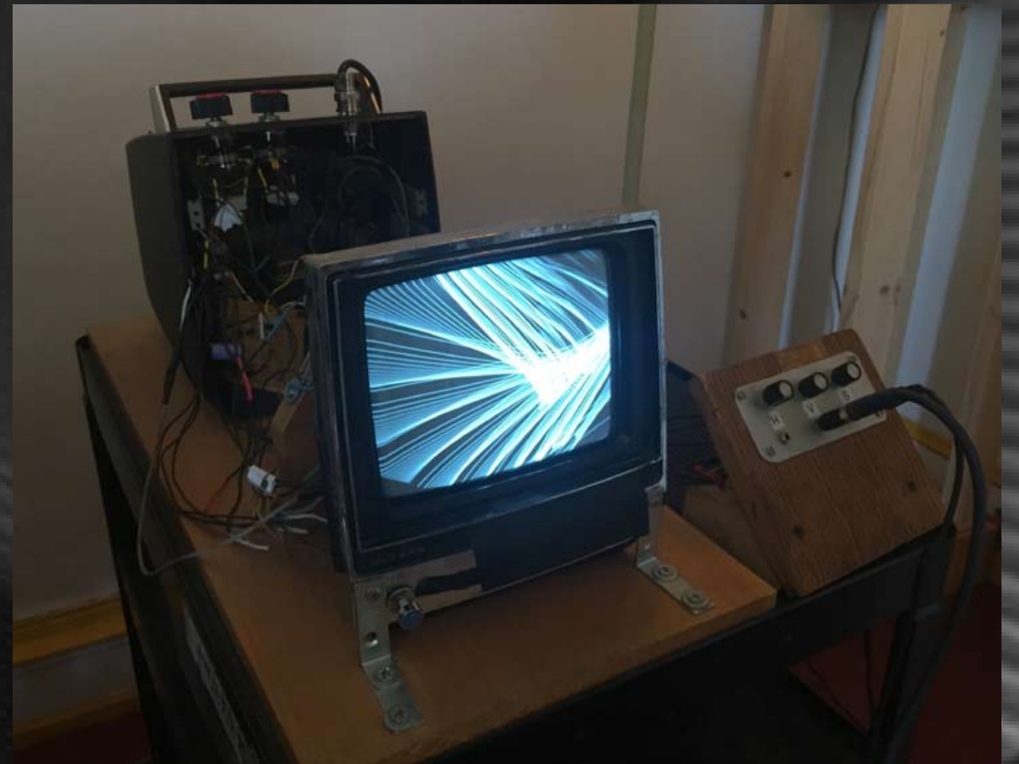
Wobbulator (Jones Raster Manipulation Unit). SC, Owego, NY., USA.
